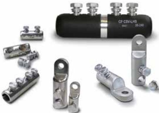
BBC Cellpack screw connectors and screw cable lugs are suitable for cross-section ranges, reliable termination and joints of both, copper and aluminium cables. Furthermore, the innovative shear-off head bolts are designed for the use of just one conventional tool. The integrated centering and further technical optimizations allow to eliminate common assembly errors already before the installation.
