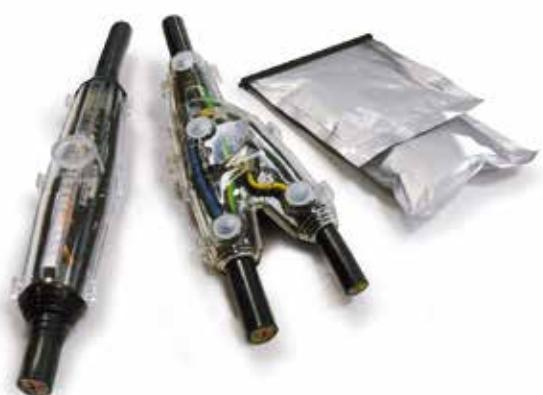
BBC Cellpack cast resin joints offer an overall long-term protection in terms of insulation values and resistance for all kind of cable accessories and cross sections. This is guaranteed by high-grade, unfilled two-component PUR cast resins which are designed for various applications as well as by the shockproof plastic moulds available with or without integrated strain relief. After the hardening process, the cable joints are resistant to mechanical and electrical loads.
