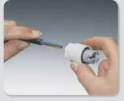
Lead the cores into the marked core entries and cut off the projecting core ends flush, i.e. so that there is no overhang.
