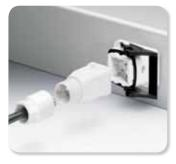
Thanks to insulation displacement connection it now only takes a few seconds to connect the 4-pole round conductor: Only the sleeve nut has to be slid onto the conductor - since splicing ring, seal and strain relief are included in the sleeve nut.
